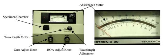
The Spectronic 20 spectrophotometer is a very important and useful scientific tool allowing you to measure the absorption patterns of individual pigments and combinations of pigments in solution. The Spectronic 20 requires care and consideration during its use.
